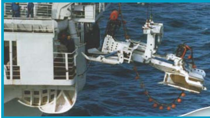
Plate 2.27 Cable plough behind tow vessel
