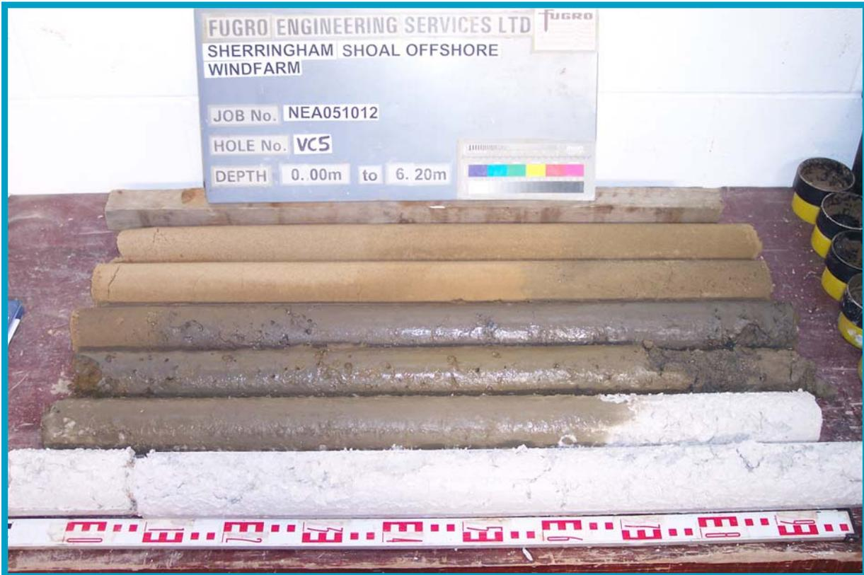
*Plate 2.2 6x1m vibrocore lengths, showing sand, bolder clay then final chalk units (VC5 edge of Pollard Shoal)*
