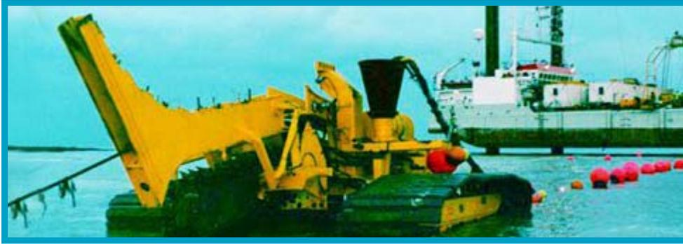
Plate 2.24 Self propelled plough
