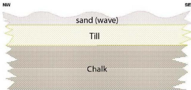
Simplified Geological cross - section across the South - East of the site. location is black line in picture (not to scale)
