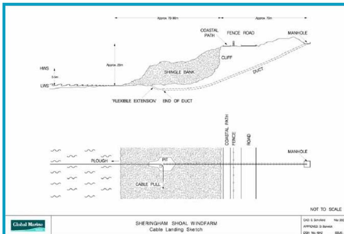
Figure 2.19 Cable Landing Illustration
