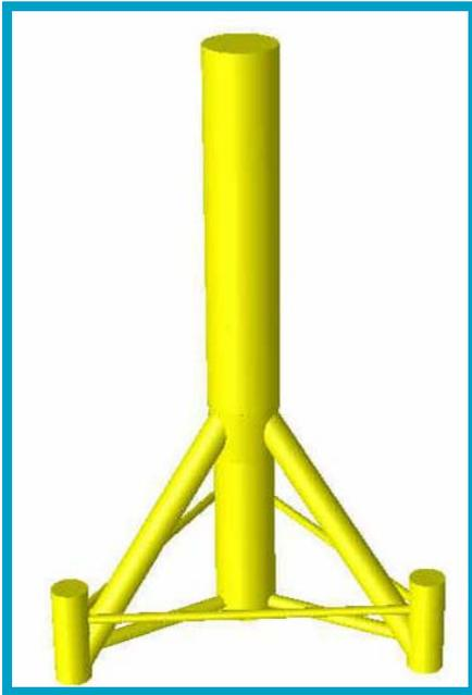
Figure 2.11 Illustration of a Tripod Foundation
