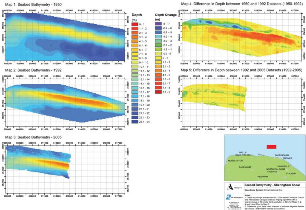
Figure 6.9 Comparison of bathymetric surveys from 1950, 1992 and 2005
