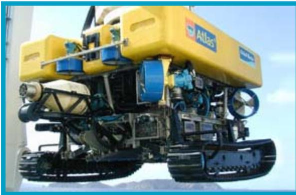
Plate 2.25 Jet equipped remotely operated vehicle
