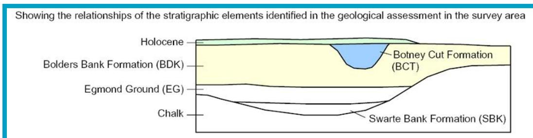
Figure 15.4 Schematic illustration of stratigraphic elements.
