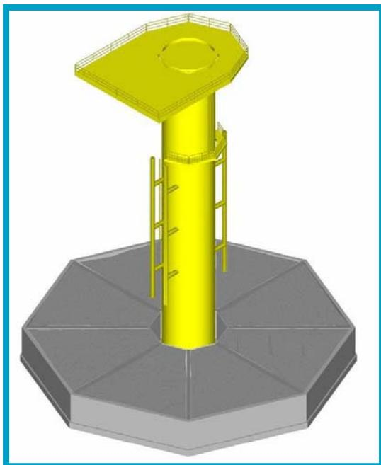
Figure 2.13 Illustrative gravity base foundation
