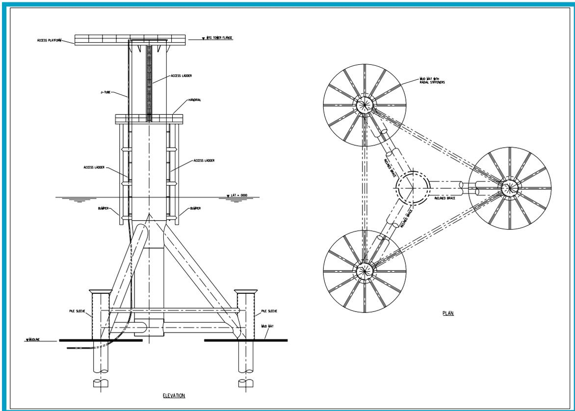
Figure 2.12 Indicative design of a tripod foundation
