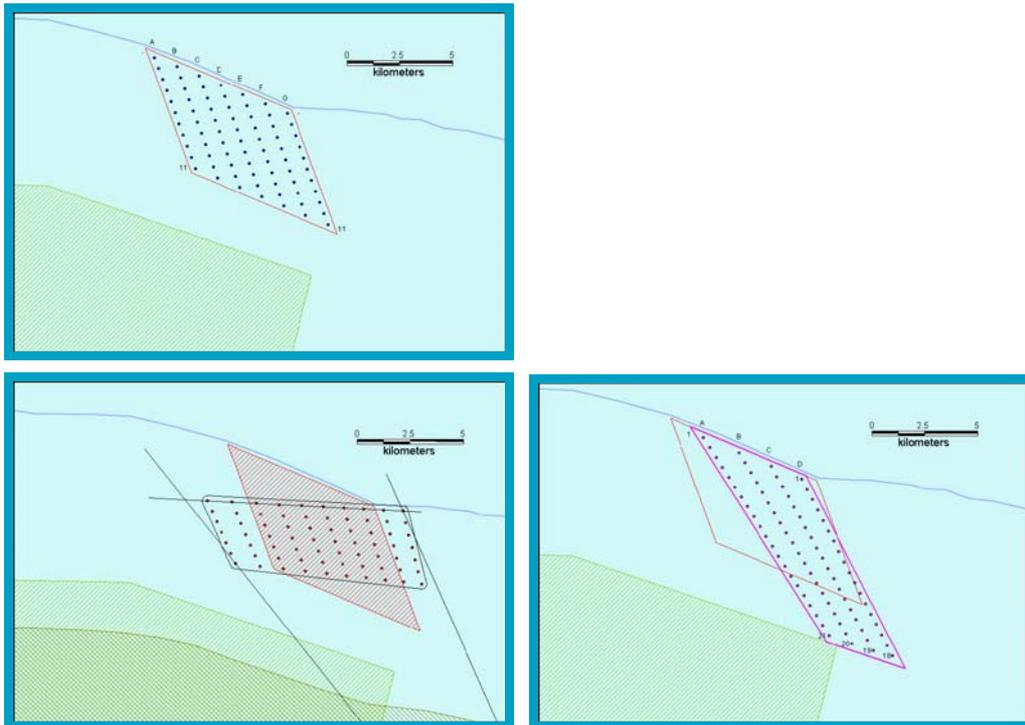
Figure 16.1 Original lay-out, stretched lay-out and radial lay-out, as assessed by QinetiQ in term of impact on clutter and shadowing. The original lay-out proves to be best.
