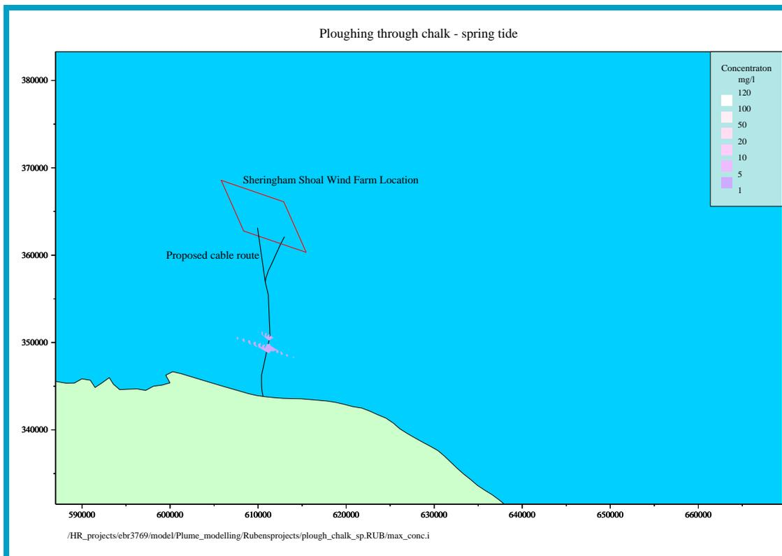
Figure 7.5 Peak suspended solids predicted to occur over spring tides for installation of export cables using the plough method
