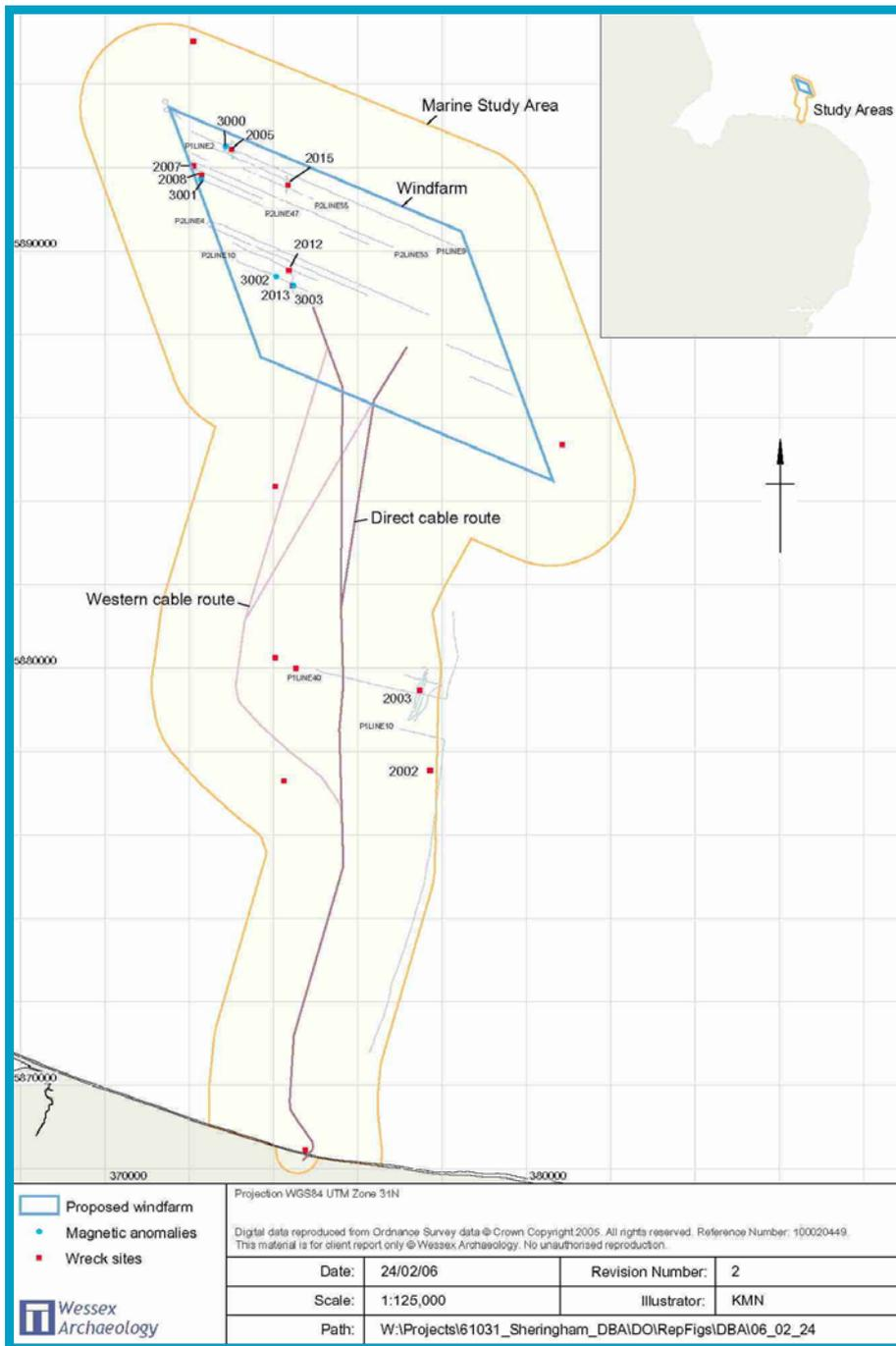
Figure 15.2 Evaluated magnetometer survey lines and magnetometer results (Source: Wessex Archaeology)
